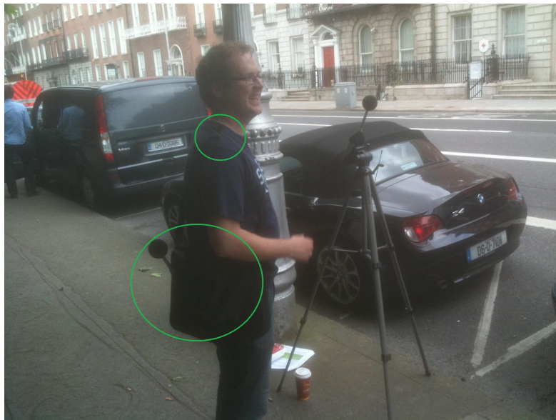
Figure 2: Test Subject. Note positioning of shoulder and waist microphones.
