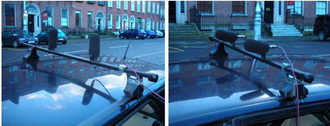
Figure 9: Microphones mounted on roof of car i) oriented upwards and ii) orientated directly into the flow.
