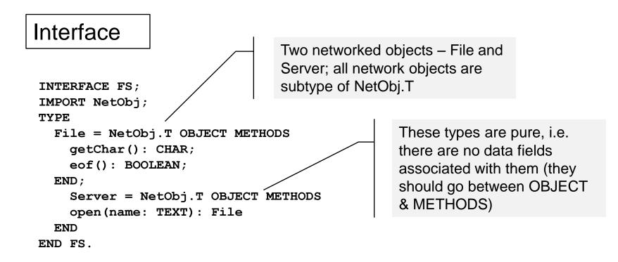
The I/F defines two network object types, one for opening files and one for reading them.
