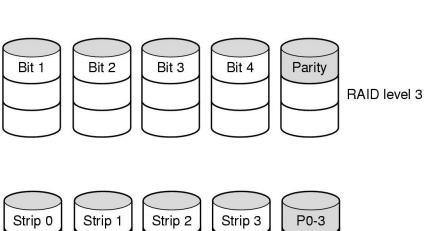
RAID 3: Bit-interleaved parity organization. If one sector is damage you know which one; used the parity to figure out what the lost bit is.
