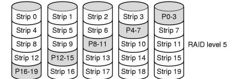
RAID 5: Block-interleaved distributed parity organization. Like 4 but distributed the parity block.
